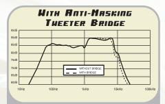
The DualMags redesigned tweeter bridge virtually eliminates woofer response irregularities. Note that the woofer's frequency response with the bridge is nearly identical to its response with no bridge at all.
