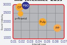
PBO provides higher sound speed and better internal loss to provide higher sound pressure level with no cone noise when compared to other fibers
