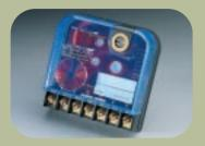
settings of tweeter attenuation either flat, -2db or -4db. The woofer can also be played full range in the low frequency or it can be crossed over to create a bandpass effect on the midrange. The crossover has a clear plastic cover so you can see all the components inside.
